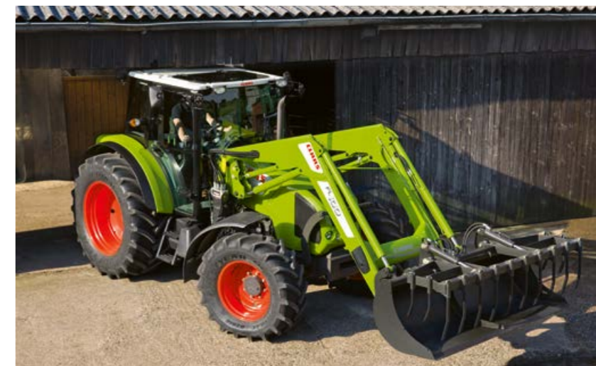
Pivoting front mudguards allow maximum steering angles.
